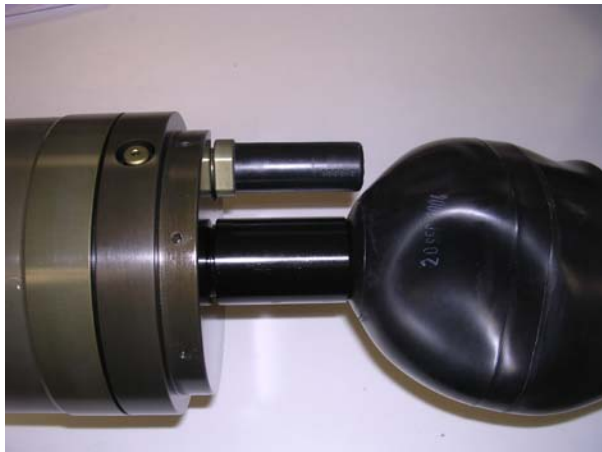
Fig 2 – Detail of lower endcap of Provor-A
